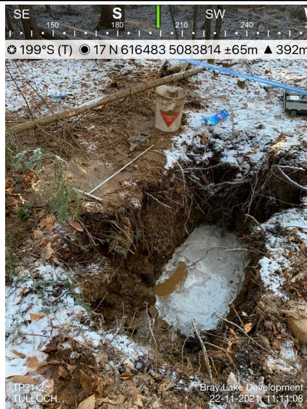
Photo 5: TP21-02 excavation note sandy soil stratum and standing water, hard surface noted at bottom of test pit.
