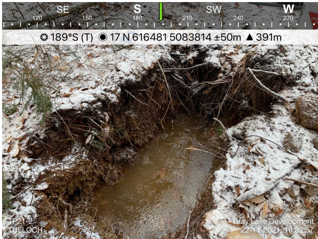
Photo 4: TP21-02 note standing water in bottom of test pit.
