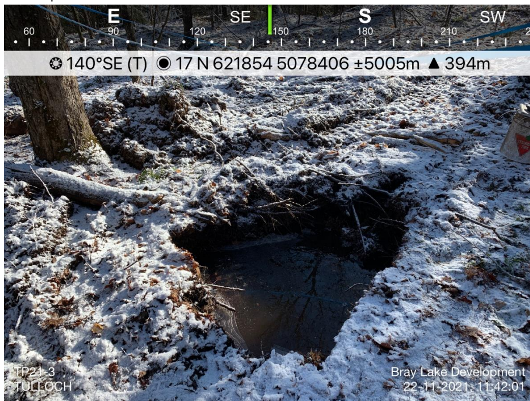
Photo 6: TP 21-03 excavation – shallow refusal at approximately 0.9 m. Excavated into hillside with visible bedrock knobs.
