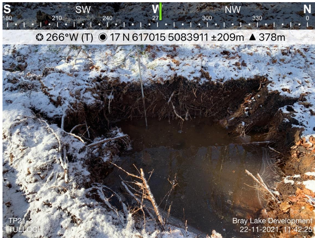
Photo 7: TP21-03 – note standing water in test pit.
